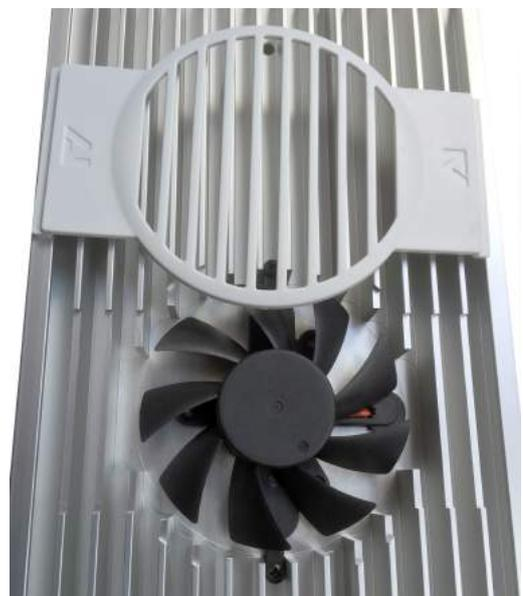
2. Now offer the bracket up to the heat sink so the lugs on the bracket slide onto the **second** inboard fin of the heat sink and carefully slide the bracket onto the light.
